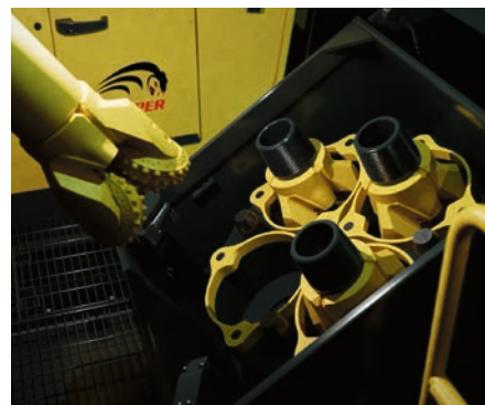
The Automatic Bit Changer for hands-free bit changes on Pit Viper drill rigs is the next step in autonomous drilling advancements. It changes rotary bits faster than manual exchanges and eliminates human interaction with the drill string for a safer way to operate a drill fleet.
