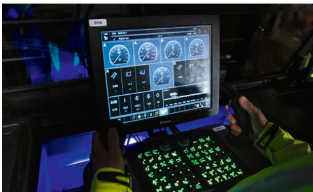
Epiroc's new Rig Control System (RCS 5) provides a number of safety and interlock features, as well as a foundation to add new functionality/options later without a major rebuild of the machine.
