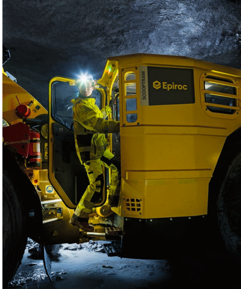
Scooptram is Epiroc's name for underground loaders. The range covers ST2-ST18, where the number indicates the tonnes of rock the bucket can carry. Several of the loaders are available in battery- and cable electric versions. Other versions are also available, for example the ST1030, our most sold loader.
