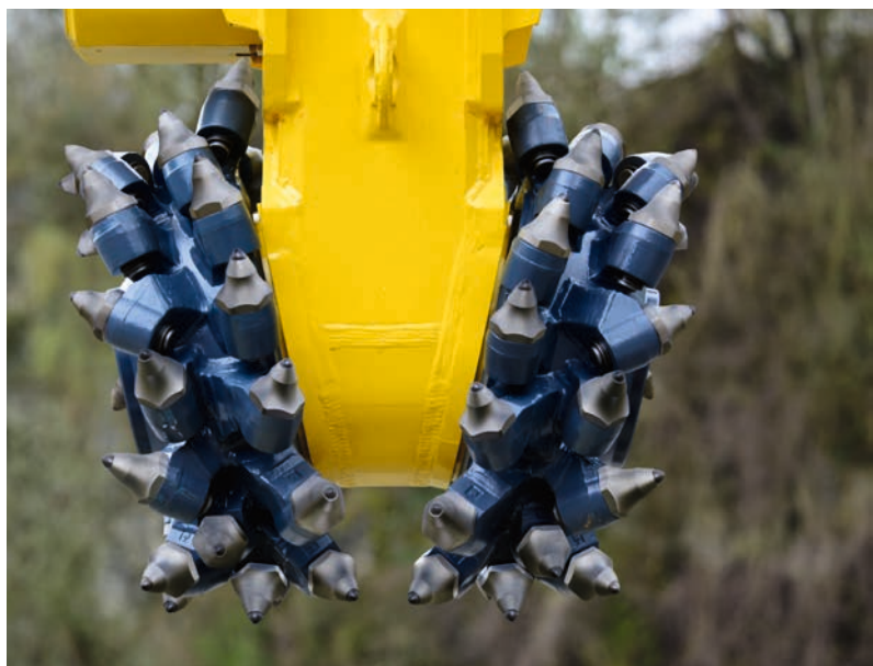
The V-shape in the V Cutter enables a cut with a flat base with no material left untouched between the drums, which means faster and more accurate trenching.
